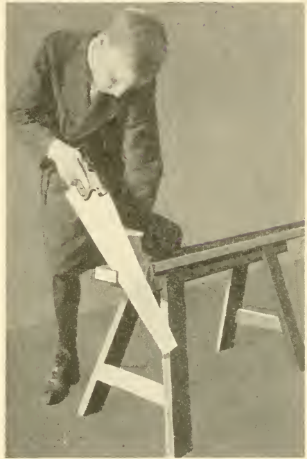
Fig. 16. Cross Sawing on a Saw Horse.
